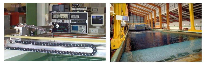
Length : 4 m Width : 2.5 m Depth : 2 m Frequency range : [8 kHz, 1.2 MHz]
